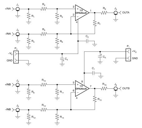
Figure 2. Schematic for DEM-OPA-MSOP-2A
