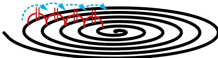
Figure 18. Parasitic Capacitive Components in an Inductor
