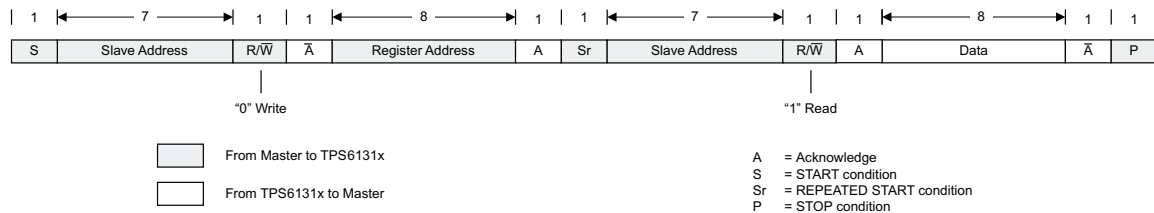
Figure 40. Read Data Transfer Format in F/S-Mode
