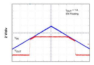
Time = 40 μs/div Figure 21. Low Dropout Start Up and Shutdown
