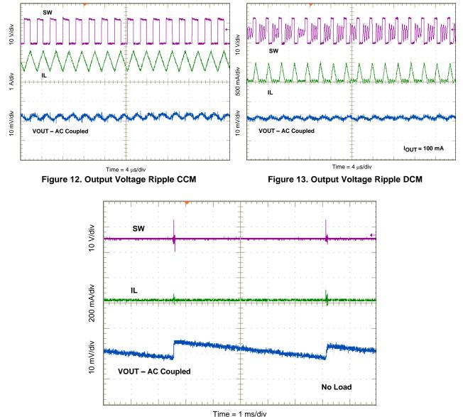
Figure 14. Output Voltage Ripple Eco-mode
