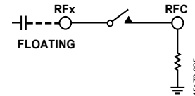
Figure 54. Series Capacitor Directly Connected to MEMS Switch
