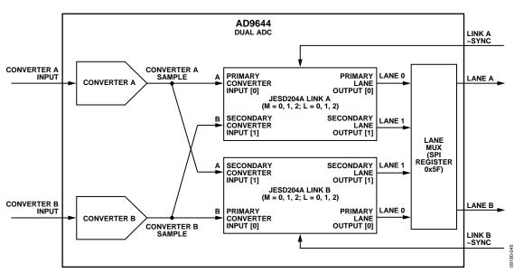
Figure 62. AD9644 Transmit Link Simplified Block Diagram
