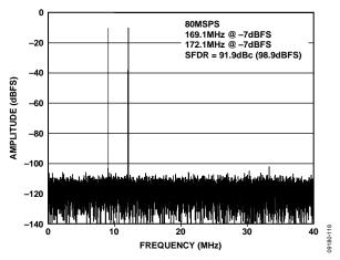
Figure 18. AD9644-80 Two-Tone FFT with  $f_{\rm IN1}$  = 169.1 MHz and  $f_{\rm IN2}$  = 172.1 MHz
