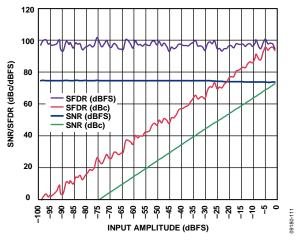
Figure 11. AD9644-80 Single-Tone SNR/SFDR vs. Input Amplitude (A<sub>IN</sub>) with  $f_{IN} = 10.1$  MHz,  $f_S = 80$  MSPS
