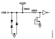
Figure 46. Equivalent CSB Input Circuit
