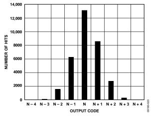
Figure 20. AD9644-80 Grounded Input Histogram
