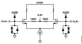
Figure 42. Equivalent Clock Input Circuit
