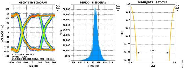
Figure 69. AD9644-155 Digital Outputs Data Eye, Histogram and Bathtub, External 100  $\Omega$  Terminations
