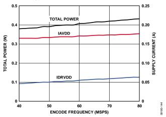
Figure 60. AD9644-80 Power and Current vs. Encode Frequency with  $f_{\rm IN}$  = 10.1 MHz
