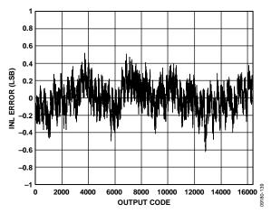
Figure 39. AD9644-155 INL with  $f_{IN} = 30.3 \text{ MHz}$
