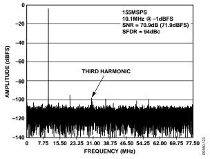
Figure 23. AD9644-155 Single-Tone FFT with  $f_{IN} = 10.1 \text{ MHz}$
