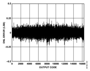
Figure 40. AD9644-155 DNL with  $f_{IN} = 30.3 \text{ MHz}$
