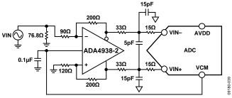
Figure 49. Differential Input Configuration Using the ADA4938-2
