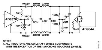
Figure 52. Differential Input Configuration Using the AD8376 (Filter Values Shown Are for a 20 MHz Bandwidth Filter Centered at 140 MHz)
