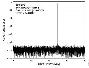
Figure 8. AD9644-80 Single-Tone FFT with  $f_{IN} = 140.1 \text{ MHz}$
