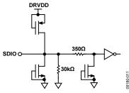
Figure 44. Equivalent SDIO Circuit
