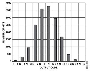
Figure 38. AD9644-155 Grounded Input Histogram
