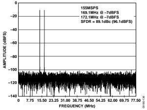
Figure 36. AD9644-155 Two-Tone FFT with  $f_{\rm IN1}$  = 169.1 MHz and  $f_{\rm IN2}$  = 172.1 MHz
