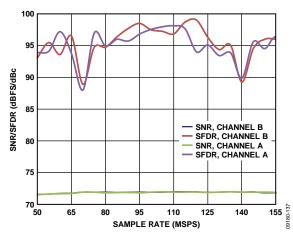
Figure 37. AD9644-155 Single-Tone SNR/SFDR vs. Sample Rate ( $f_s$ ) with  $f_{\rm IN}$  = 70. MHz
