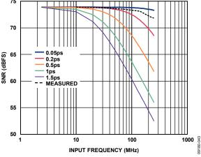
Figure 59. SNR vs. Input Frequency and Jitter
