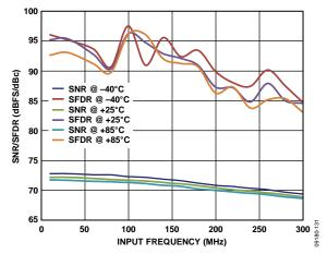
Figure 31. AD9644-155 Single-Tone SNR/SFDR vs. Input Frequency ( $f_{\rm IN}$ ) and Temperature with 1.75 V p-p Full-Scale,  $f_{\rm S}=80$  MSPS
