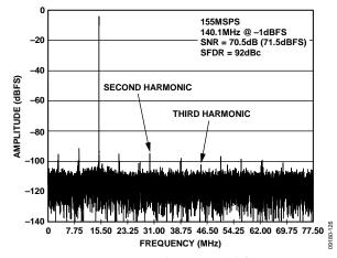
Figure 26. AD9644-155 Single-Tone FFT with  $f_{IN} = 140.1$  MHz
