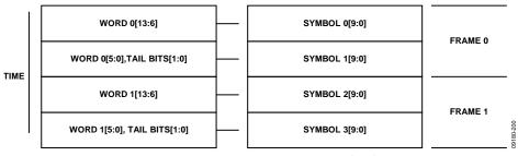
Figure 64. AD9644 14-Bit Data Transmission with Tail Bits
