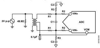
Figure 50. Differential Transformer-Coupled Configuration
