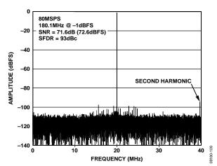
Figure 9. AD9644-80 Single-Tone FFT with  $f_{IN} = 180.1$  MHz
