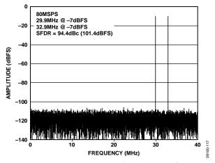
Figure 17. AD9644-80 Two-Tone FFT with  $f_{IN1} = 29.9$  MHz and  $f_{IN2} = 32.9$  MHz
