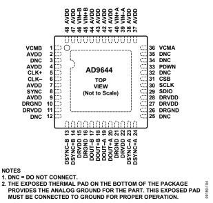
Figure 4. LFCSP Pin Configuration (Top View)
