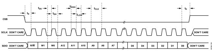
Figure 71. Serial Port Interface Timing Diagram
