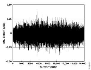
Figure 22. AD9644-80 DNL with  $f_{IN} = 30.3 \text{ MHz}$
