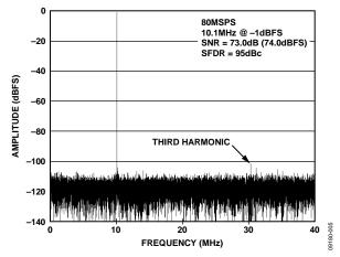
Figure 5. AD9644-80 Single-Tone FFT with  $f_{IN} = 10.1 \text{ MHz}$
