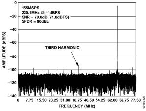
Figure 28. AD9644-155 Single-Tone FFT with  $f_{IN}$  = 220.1 MHz
