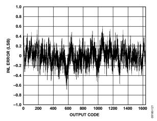
Figure 21. AD9644-80 INL with  $f_{IN} = 30.3 \text{ MHz}$
