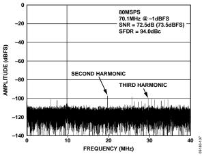
Figure 7. AD9644-80 Single-Tone FFT with  $f_{IN} = 70.1 \text{ MHz}$
