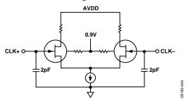
Figure 53. Equivalent Clock Input Circuit
