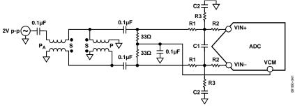
Figure 51. Differential Double Balun Input Configuration
