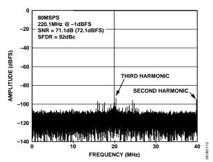
Figure 10. AD9644-80 Single-Tone FFT with  $f_{IN}$  = 220.1 MHz
