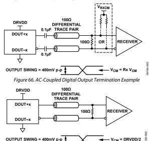
Figure 67. DC-Coupled Digital Output Termination Example
