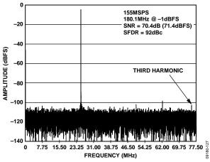
Figure 27. AD9644-155 Single-Tone FFT with  $f_{IN} = 180.1$  MHz
