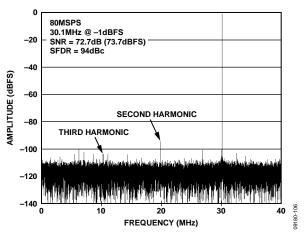
Figure 6. AD9644-80 Single-Tone FFT with  $f_{IN} = 30.1 \text{ MHz}$
