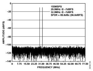
Figure 35. AD9644-155 Two-Tone FFT with  $f_{IN1} = 29.9$  MHz and  $f_{IN2} = 32.9$  MHz
