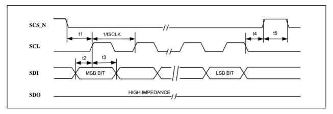
FIGURE 6-10: SPI DATA OUTPUT TIMING
