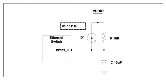
Figure 7-2 illustrates a reset circuit recommended for applications where reset is driven by another device, such as a CPU. At power-on reset, R, C and D1 provide the necessary ramp rise time to reset the KSZ9893R. The RST\_OUT\_N from the CPU provides a warm reset after power-up.
