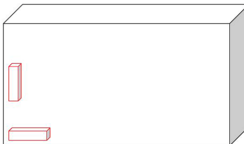
Figure 2-2. Actuator Mounting Locations in Handheld Devices
