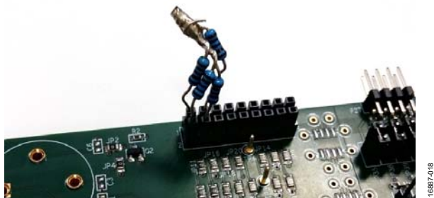
Figure 19. 1 k \Omega Resistor Star Connected on P5
