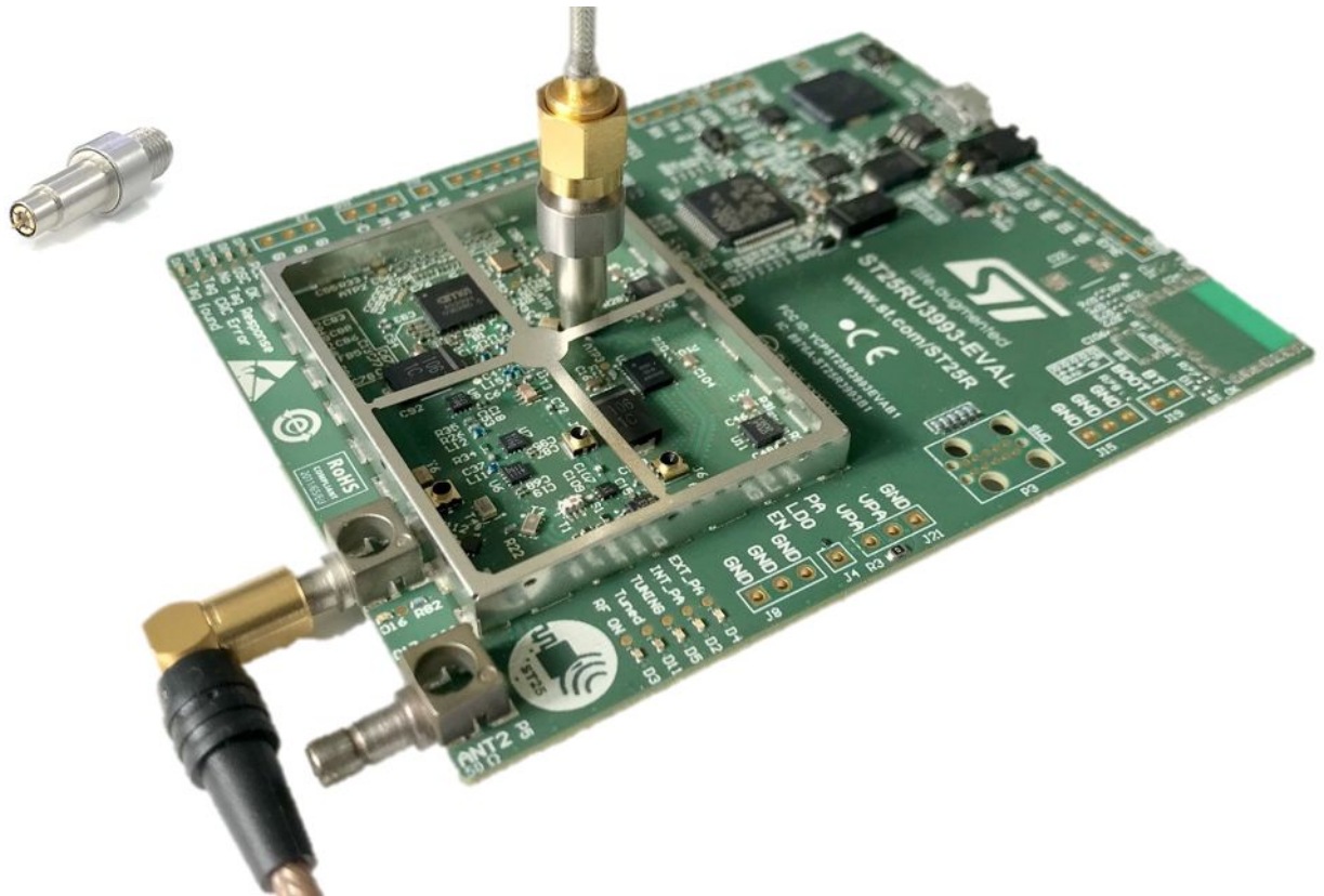
Figure 12. Connecting to the RF test points with the SMB adapter
