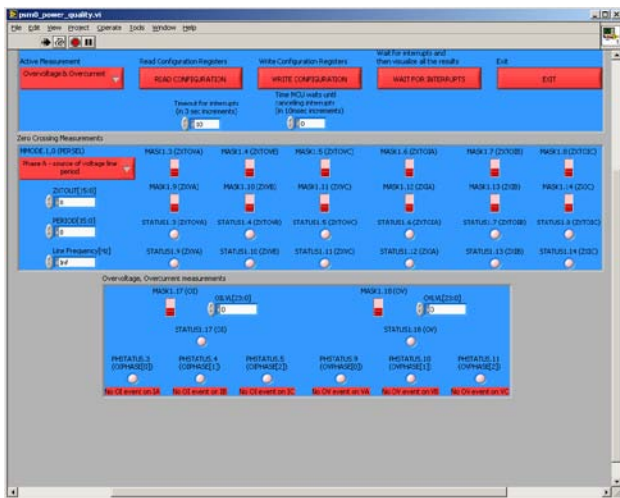
Figure 23. Overvoltage and Overcurrent Measurements Panel
