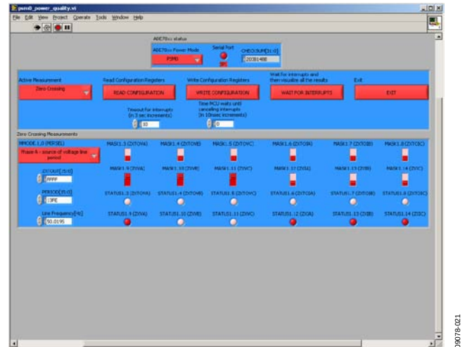
Figure 21. Power Quality Zero-Crossing Measurements Panel
