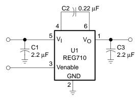
For all necessary signals there are single-pin connectors on the board. To operate the board, connect a power source with the appropriate voltage level between  $V_{\mbox{\footnotesize{IN}}}$  and GND.
