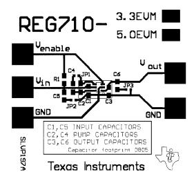
Figure 2–3 shows the metal layer of the board.
