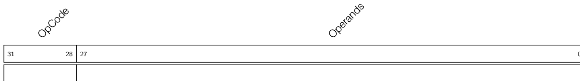
Figure 30-6. ULP-FSM Instruction Format
