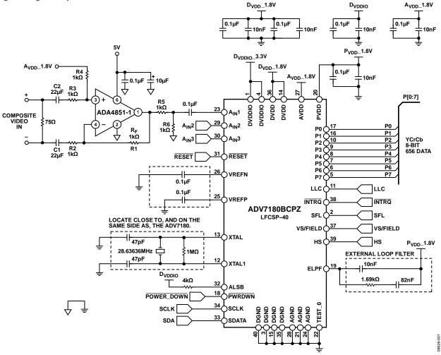
Figure 1. Low Cost Differential Video Receiver Using the ADA4851-1 (Simplified Schematic: Decoupling and All Connections Not Shown)
