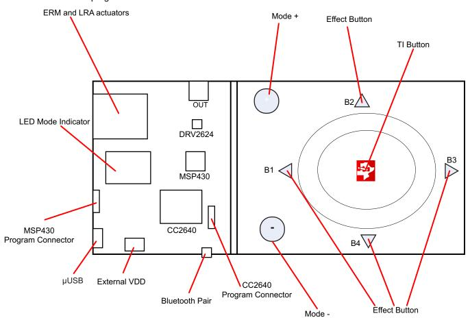
Figure 2. Board Diagram
