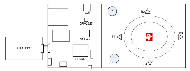
Figure 17. FET Programmer Connection
