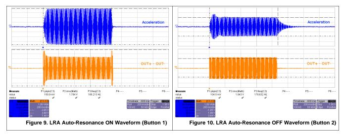
The reason for higher acceleration can be seen in the acceleration versus frequency graph below. The LRA has a very narrow operating frequency range due to the properties of a spring-mass system. Furthermore, the resonance frequency drifts over various conditions such as temperature and drive voltage. With the Smart Loop auto-resonance feature, the DRV2624 dynamically tracks the exact resonant frequency to maximize the vibration force.
