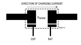
Figure 12. Kelvin Sensing of Charging Current
