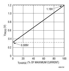
Figure 2. V<sub>PROG</sub> vs I<sub>CHARGE</sub>
