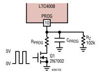
Figure 5. PWM Current Programming
