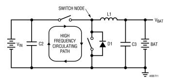
Figure 11. High Speed Switching Path
