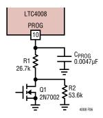
Figure 6. 2-Level Current Programming
