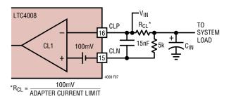
Figure 7. Adapter Current Limiting
