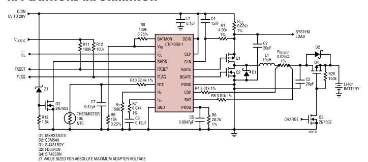
Figure 10. Typical LTC4008-1 Application (12.3V/4A)
