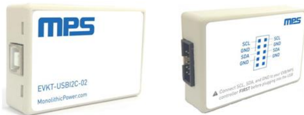
Figure 3: EVKT-USBI2C-02 Communication Interface
