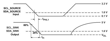
Figure 8. Sink Side Output AC Measurements
