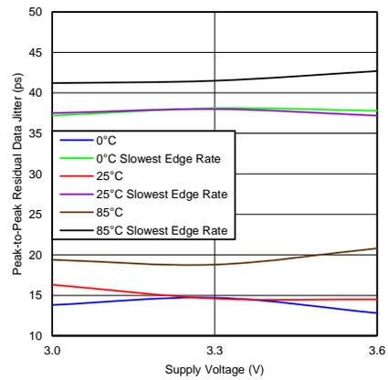
Figure 16. Residual Jitter of 3 Gbps vs Supply Voltage
