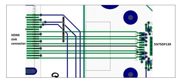
Figure 36. Sink Side Layout Example
