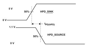
Figure 4. HPD Timing Diagram (HPDINV = HIGH)
