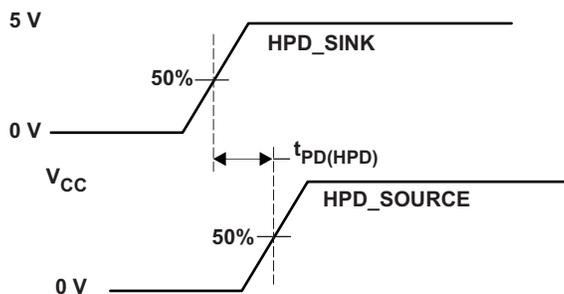
Figure 3. HPD Timing Diagram (HPDINV = LOW)
