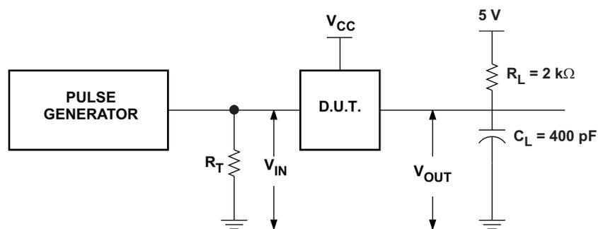
**Figure 6. Sink Side Test Circuit (SCL\_SINK, SDA\_SINK)**
