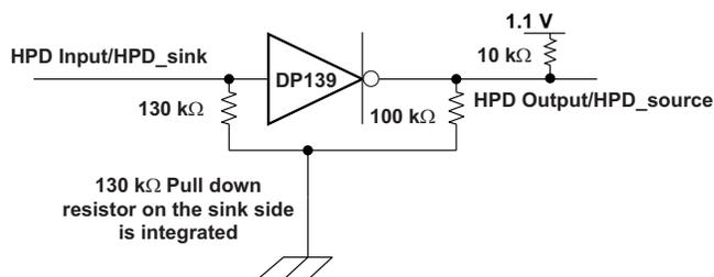
Figure 2. HPD Test Circuit (VOH = 1.1), HPDINV = HIGH
