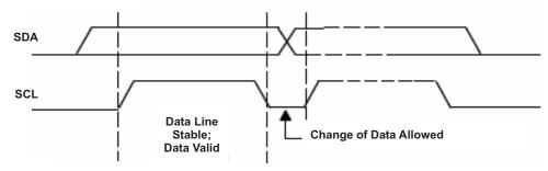
Figure 27. I<sup>2</sup>C Bit Transfer
