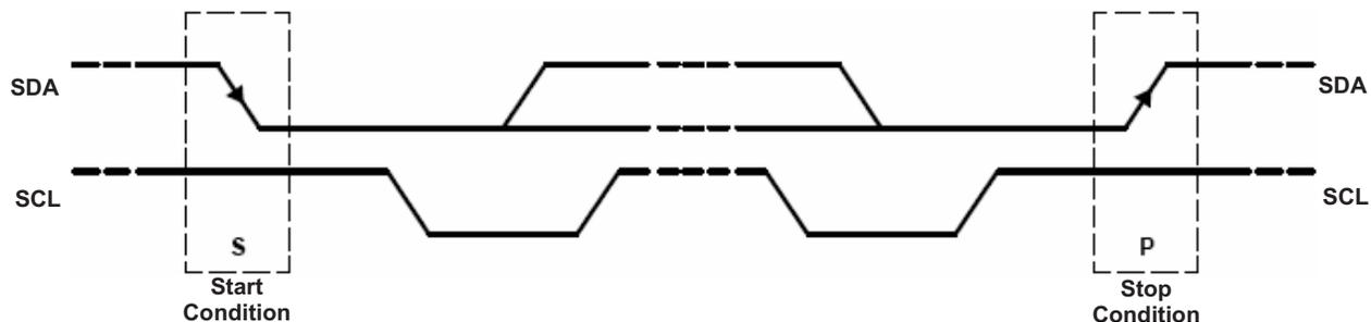
**Figure 26. I<sup>2</sup>C Start And Stop Conditions**
