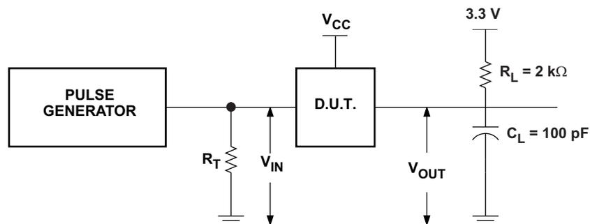
**Figure 5. Source Side Test Circuit (SCL\_SOURCE, SDA\_SOURCE)**
