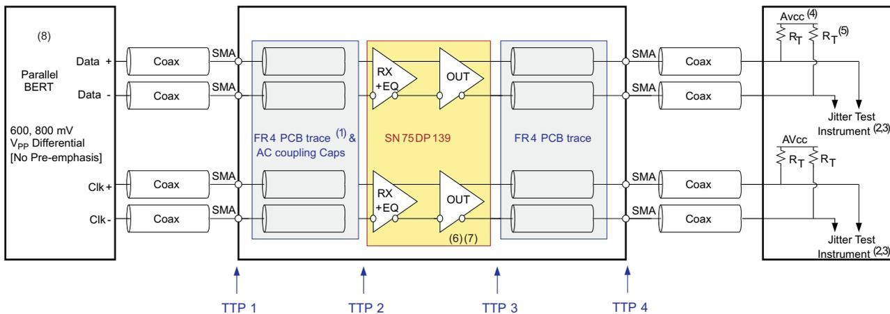
1. The FR4 trace between TTP1 and TTP2 is designed to emulate 1-8" of FR4, AC coupling cap, connector and another 1-8" of FR4. Trace width - 4 mils.
