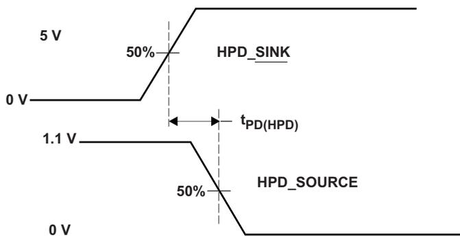
Figure 4. HPD Timing Diagram (HPDINV = HIGH)
