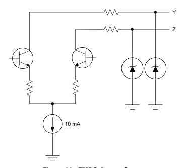
Figure 22. TMDS Output Stage
