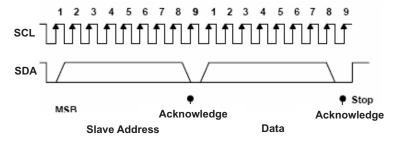
Figure 29. I<sup>2</sup>C Address And Data Cycles
