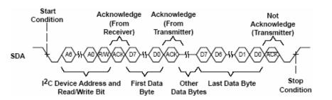
Figure 31. Multiple Byte Read Transfer
