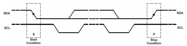
Figure 26. I<sup>2</sup>C Start And Stop Conditions
