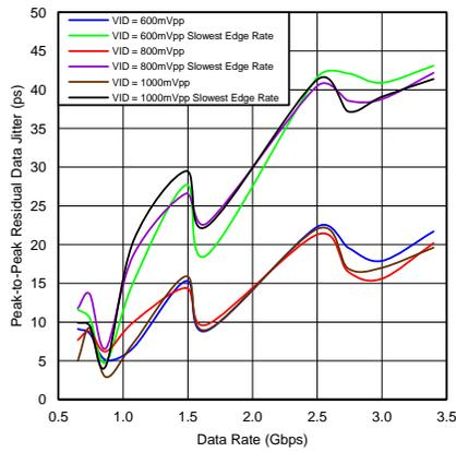
Figure 17. Residual Jitter vs Data Rate (RGZ Package)
