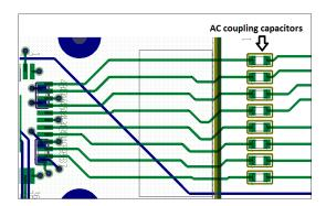
Figure 37. AC Capacitors Placement and Routing Example
