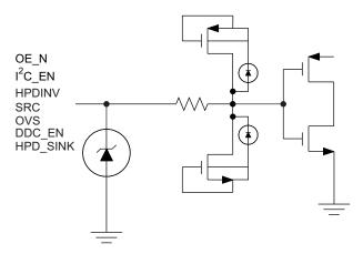
Figure 23. HPD and Control Input Stage
