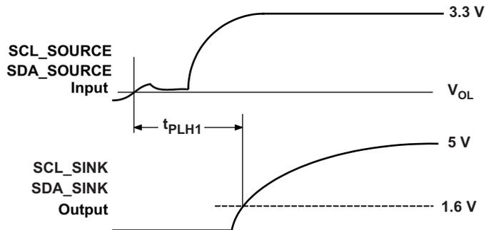
Figure 9. Sink Side Output AC Measurements Continued
