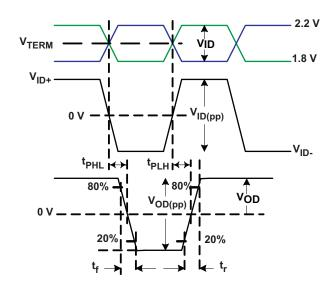
Figure 11. TMDS Main Link Timing Measurements
