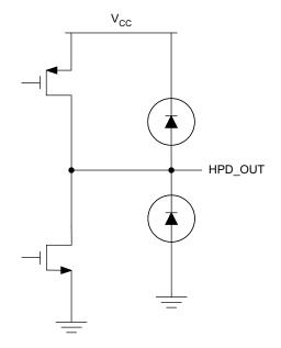
Figure 24. HPD Output Stage
