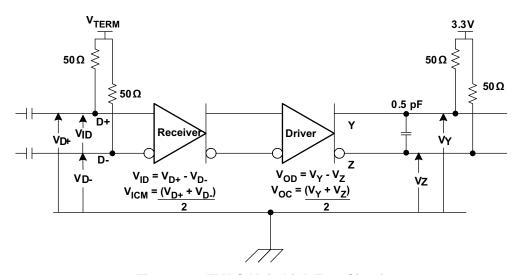
Figure 10. TMDS Main Link Test Circuit
