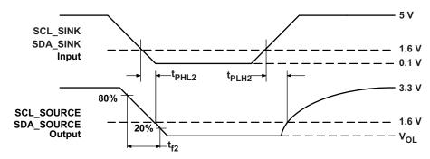
Figure 7. Source Side Output AC Measurements
