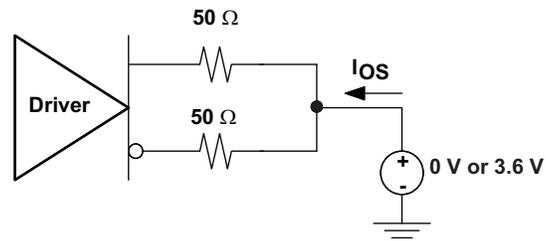
**Figure 14. TMD5 Main Link Short Circuit Output Circuit**
