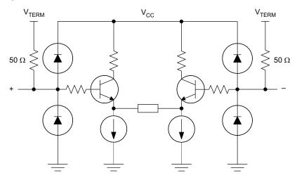
Figure 21. DisplayPort Input Stage
