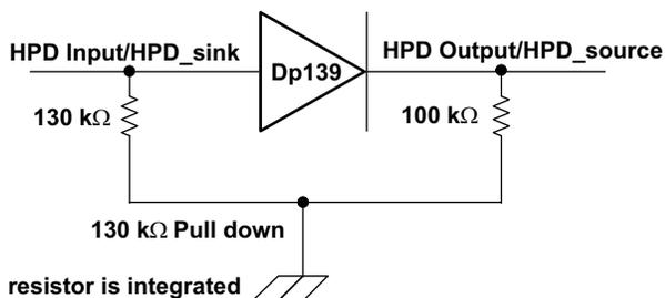
Figure 1. HPD Test Circuit (HPDINV = LOW)
