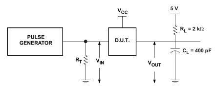
Figure 6. Sink Side Test Circuit (SCL\_SINK,SDA\_SINK)
