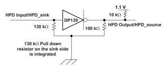
Figure 1. HPD Test Circuit (HPDINV = LOW)
