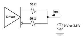
Figure 14. TMDS Main Link Short Circuit Output Circuit
