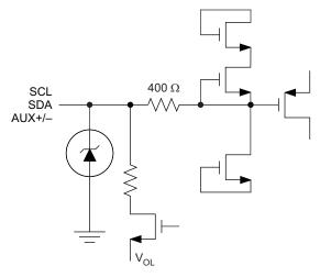
Figure 25. I<sup>2</sup>C Input and Output Stage
