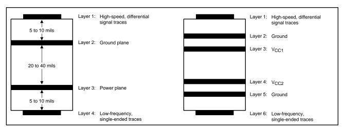
Figure 34. Recommended 4- or 6- Layer (0.062") Stack for a Receiver PCB Design
