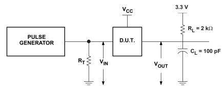
Figure 5. Source Side Test Circuit (SCL\_SOURCE, SDA\_SOURCE)
