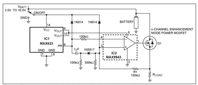
Figure 1. This logic-controlled switch circuit provides short-circuit protection at R<sub>LOAD</sub>.
