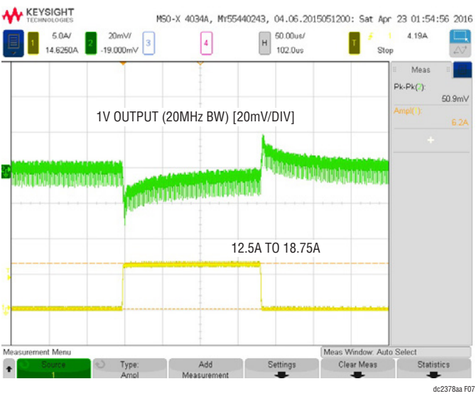
Figure 7. Measured Channel 2 12.5A to 18.75A Load Transient ( V_{IN} = 12V , V_{OUT2} = 1V )
