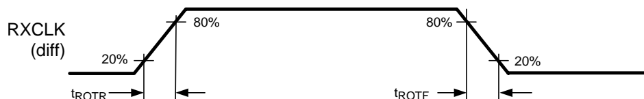
Figure 4. LVDS Output Transition Time
