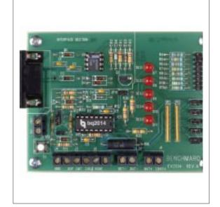
The menu-driven software provided with the EV2014 displays charge/discharge activity and allows user interface to the bq2014 from any standard DOS PC.
