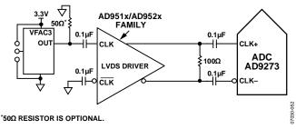
Figure 57. Differential LVDS Sample Clock
