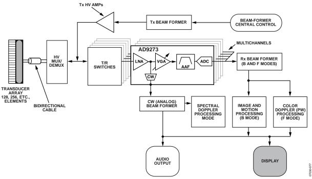
Figure 37. Simplified Ultrasound System Block Diagram
