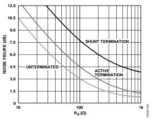
Figure 42. Noise Figure vs.  $R_s$  for Shunt Termination, Active Termination Matched, and Unterminated Inputs,  $V_{GAIN} = 0.8 V$
