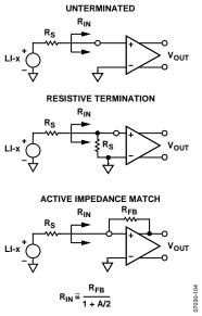
Figure 41. Input Configurations
