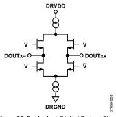
Figure 29. Equivalent Digital Output Circuit
