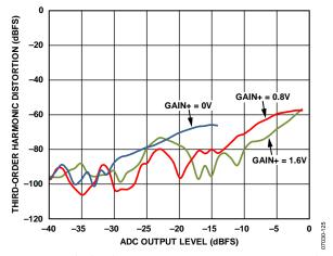
Figure 22. Third-Order Harmonic Distortion vs. ADC Output Level
