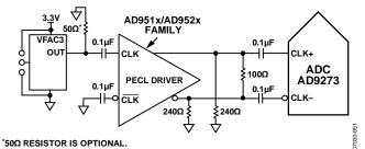
Figure 56. Differential PECL Sample Clock
