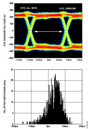
Figure 65. Data Eye for LVDS Outputs in ANSI-644 Mode with Trace Lengths of Less than 24 Inches on Standard FR-4
