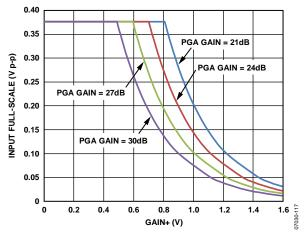
Figure 48. LNA with 15.6 dB Gain Setting/VGA Full-Scale Limitations
