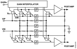
Figure 51. Simplified VGA Schematic
