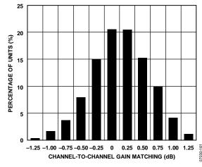
Figure 11. Gain Match Histogram, GAIN+ = 1.3 V
