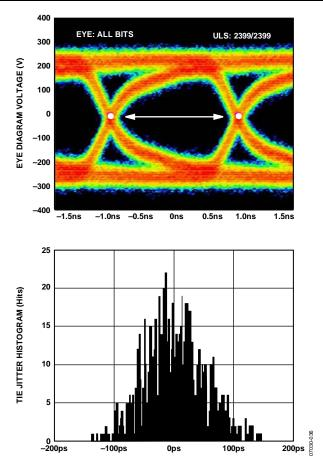
Figure 66. Data Eye for LVDS Outputs in ANSI-644 Mode with Trace Lengths of Greater than 24 Inches on Standard FR-4
