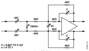
Figure 54. Simplified Filter Schematic
