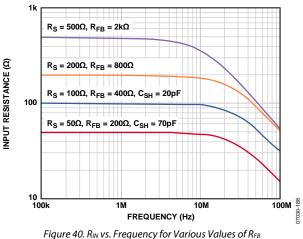
Figure 40.  $R_{IN}$  vs. Frequency for Various Values of  $R_{FB}$ (Effects of  $R_s$  and  $C_{SH}$  Are Also Shown)
