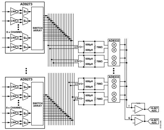
Figure 45. Typical Connection Interface with the AD8333 or AD8339 using the CWDx± Outputs
