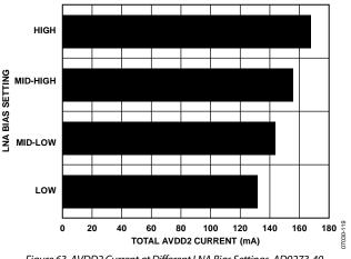
Figure 63. AVDD2 Current at Different LNA Bias Settings, AD9273-40
