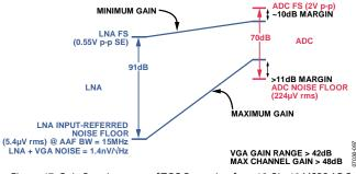
Figure 47. Gain Requirements of TGC Operation for a 12-Bit, 40 MSPS ADC
