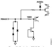
Figure 31. Equivalent RBIAS Circuit
