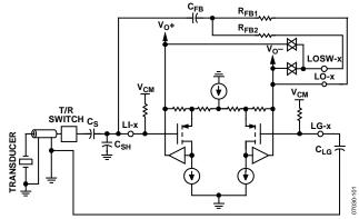
Figure 39. Simplified LNA Schematic
