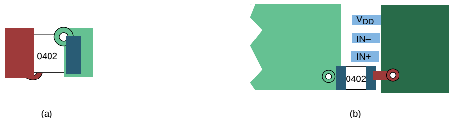
Figure 29. Typical Decoupling Capacitor Layouts
