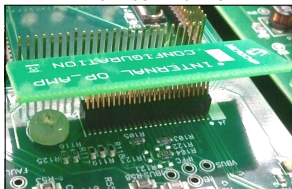
FIGURE 2: INTERNAL OP AMP CONFIGURATION BOARD
