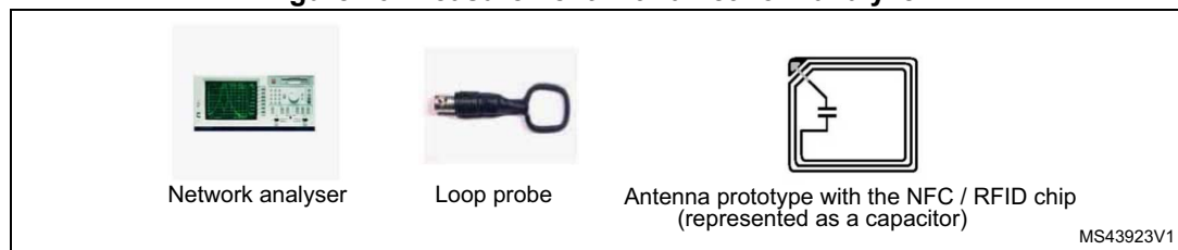
Figure 10. Measurement with a network analyzer
