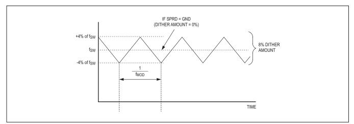
Figure 1. Frequency Spread Timing Diagram
