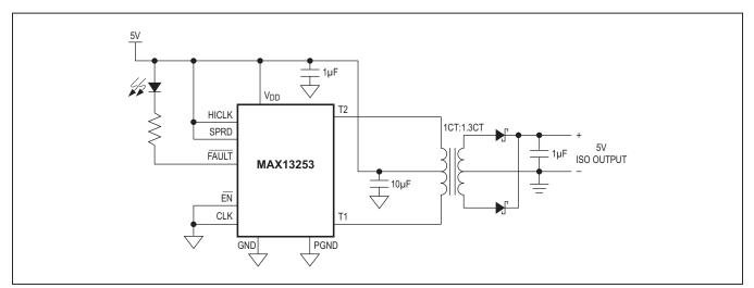
Figure 4. 5V to Isolated, Unregulated 6V Application Circuit
