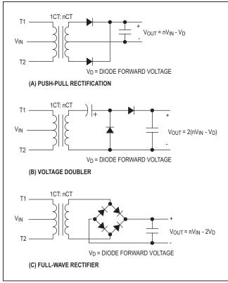
Figure 3. Secondary-Side Rectification Topologies
