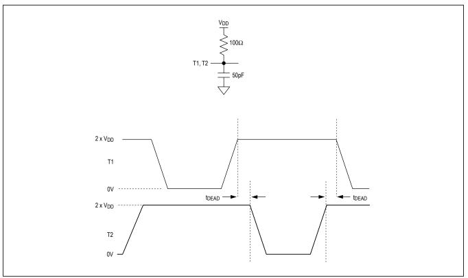
Figure 2. T1, T2 Timing Diagram
