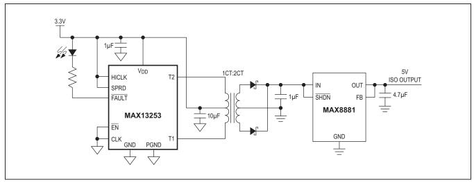
Figure 5. 3.3V to Isolated, Regulated 5V Application Circuit
