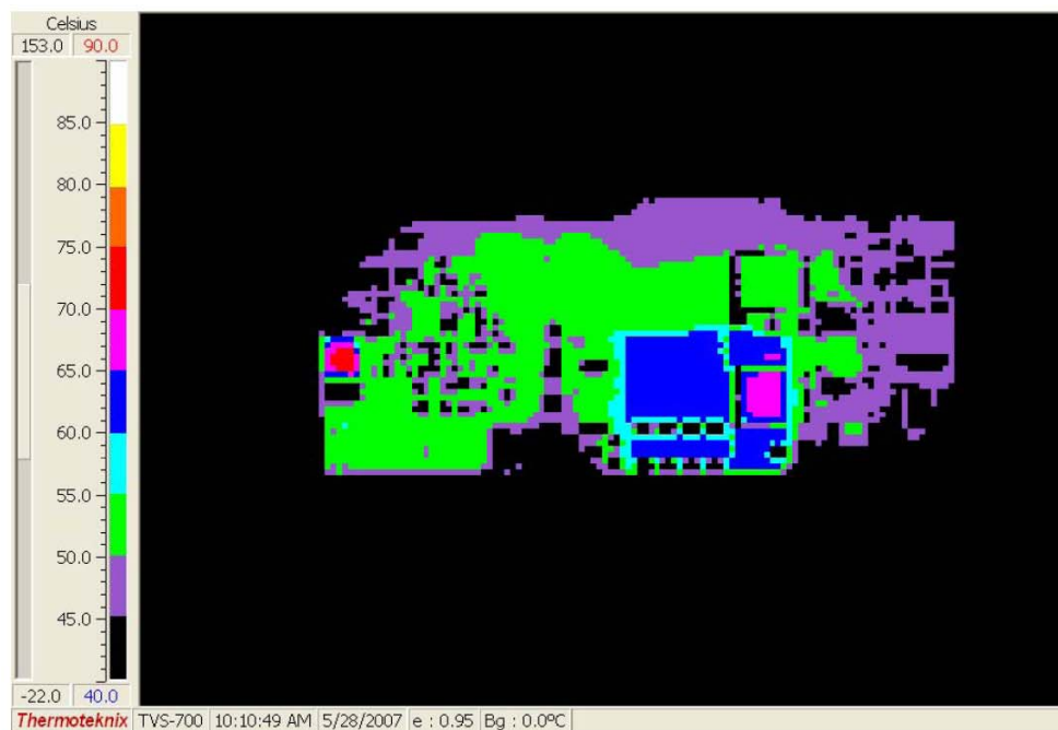
Figure 7. Thermal Map, Backside at 18Vin and 4.2Aout ( T_a = 25 degrees C)
