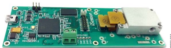
Figure 3. ADIS16448/PCBZ Installation Example
