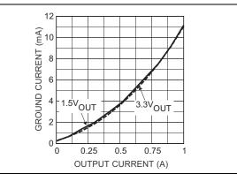
FIGURE 2-11: Ground Current vs. Output Current.
