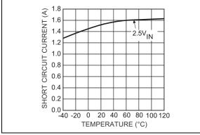
FIGURE 2-25: Short Circuit Current vs. Temperature.
