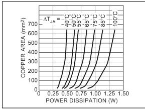
FIGURE 4-4: Copper Area vs. Power SO-8 Power Dissipation.
