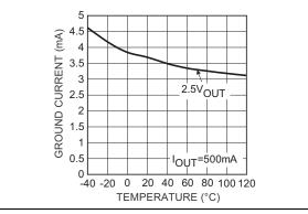
FIGURE 2-21: Ground Current vs. Temperature.
