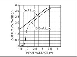
FIGURE 2-10: Dropout Characteristics (3.3V).
