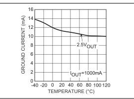
FIGURE 2-22: Ground Current vs. Temperature.
