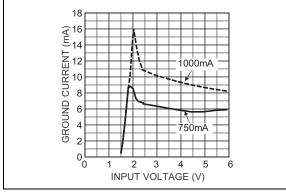
FIGURE 2-13: Ground Current vs. Supply Voltage (1.5V).
