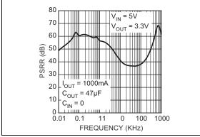
FIGURE 2-2: Power Supply Rejection Ratio.
