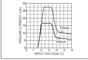
FIGURE 2-19: Ground Current vs. Supply Voltage (3.3V).
