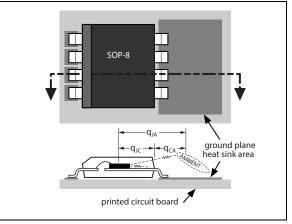
FIGURE 4-3: Thermal Resistance.
