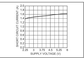
FIGURE 2-24: Short Circuit Current vs. Supply Voltage.
