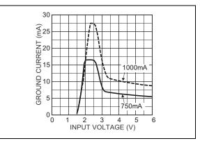
FIGURE 2-17: Ground Current vs. Supply Voltage (2.5V).
