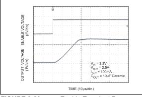
FIGURE 2-33: Enable Transient Response.
