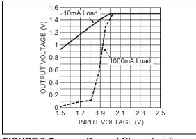
**FIGURE 2-7:** Dropout Characteristics (1.5V).
