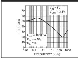
FIGURE 2-1: Power Supply Rejection Ratio.
