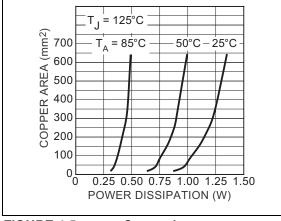
FIGURE 4-5: Copper Area vs. Power-SOIC Power Dissipation.
