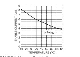
*FIGURE 2-29:* Enable Current vs. Temperature.
