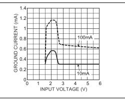
*FIGURE 2-16:* Ground Current vs. Supply Voltage (2.5V).
