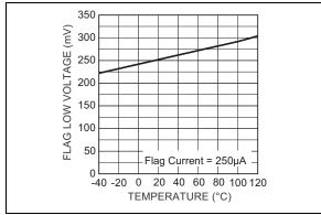
FIGURE 2-27: Flag Low Voltage vs. Temperature.
