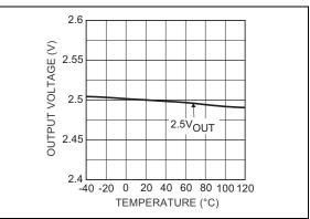
*FIGURE 2-23:* Output Voltage vs. Temperature.
