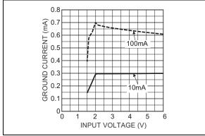
FIGURE 2-14: Ground Current vs. Supply Voltage (1.8V).
