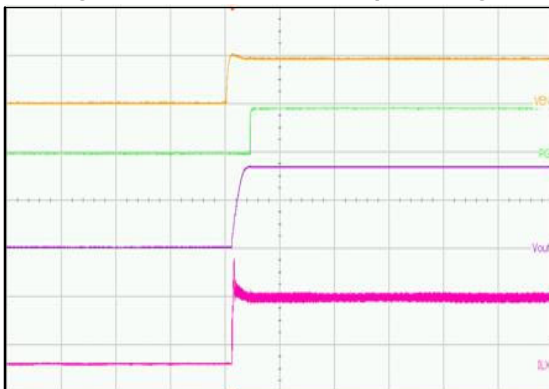
(VIN = 5 V, VOUT = 1.8 V, IOU = 3 A, no CSS) Upper Trace: Enable Pin Voltage, 5 V / div Second Trace: Power Good Pin Voltage, 5 V / div Third Trace: Output Voltage, 2 V / div Lower Trace: Inductor Current, 2 A / div Time = 2 ms / div
