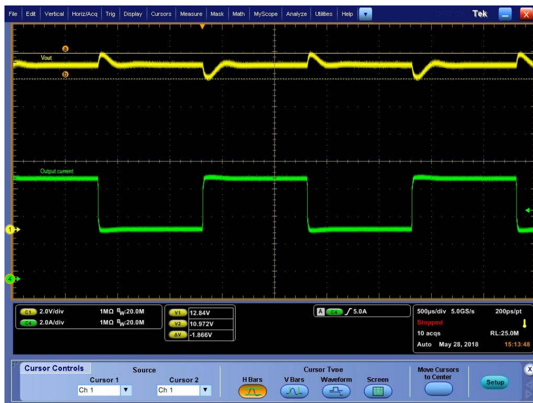
Figure 20. Load transient: I_{out}=4 to 8 A, V_{in}=48 V
