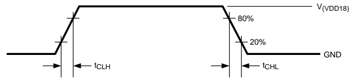
Figure 1. LVCMOS Transition Times
