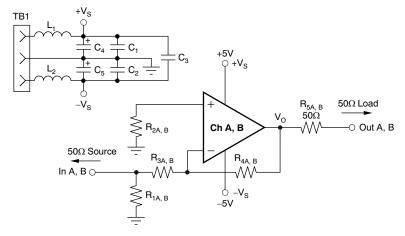
Figure 2. Schematic for DEM-OPA-SO-2C
