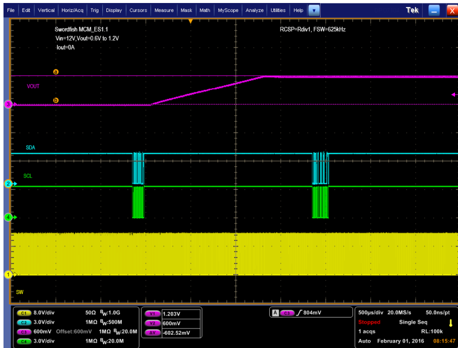
Figure 8. PMBus V_{OUT} Step-Up = 0.6 V to 1.2 V at 0 A
