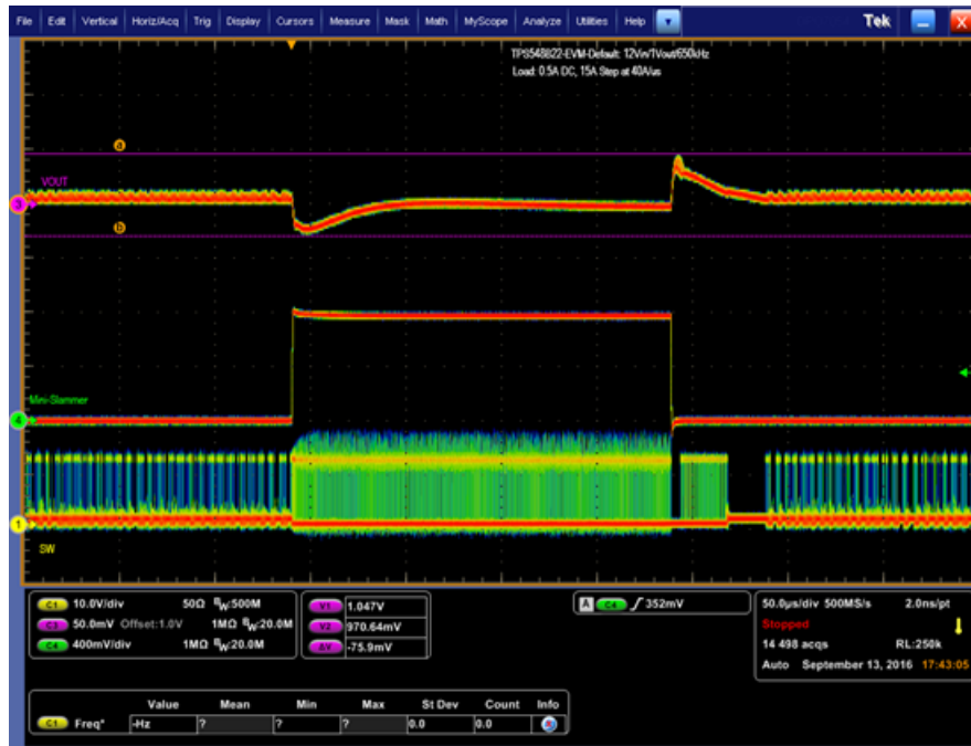
Figure 13. Transient Response of 1-V Output at 12 V IN , Transient is 0.5 A to 15.5 A, the Step is 15 A at 40 A/μs
