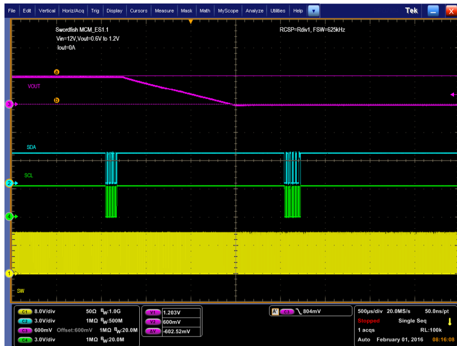
Figure 9. PMBus V OUT Step-Down = 1.2 V to 0.6 V at 0 A
