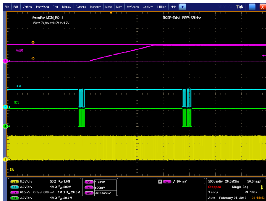
Figure 10. PMBus V OUT Step-Up = 0.6 V to 1.2 V at 25 A
