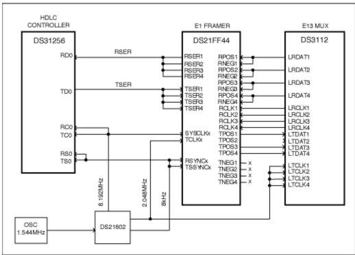
Figure 1. Example OF typical connections.
