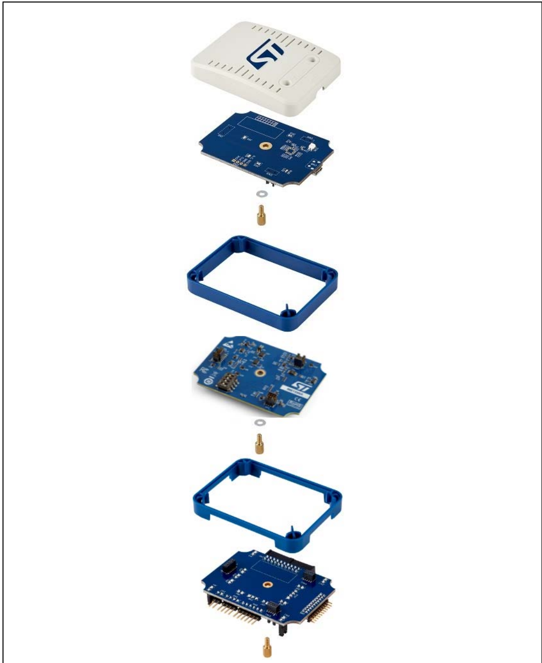
Figure 17. Opened casing for access to all connectors (through MB1440 adapter board)
