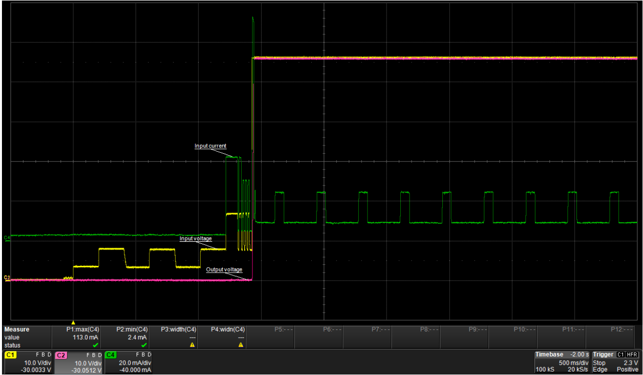
Figure 17. No Load Start-up, MPS Circuit Turned ON
