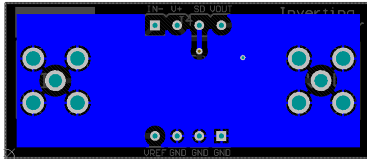
Figure 32. Inverting Comparator Bottom Layer
