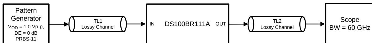
Figure 11. Test Setup Connections Diagram Pre-Channel and Post-Channel, No Tx Source De-emphasis
