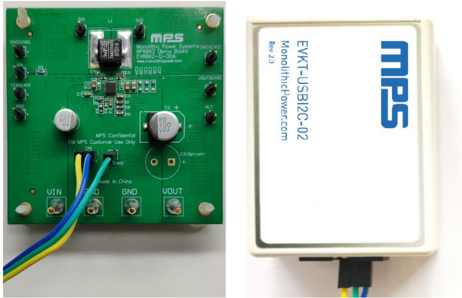
Figure 6: EVB to MPS I 2 C Communication Interface Device Wire Connection
