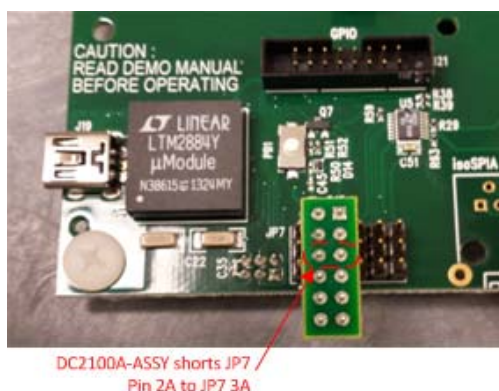
Figure 15 - JP7 Placement to Force Bootloader Mode
