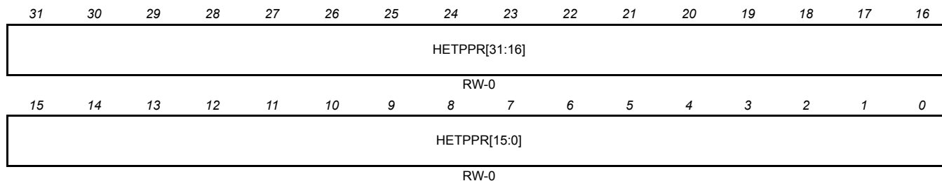
Figure 18-62. Parity Pin Register (HETPPR) [0xFFF7B87C]
