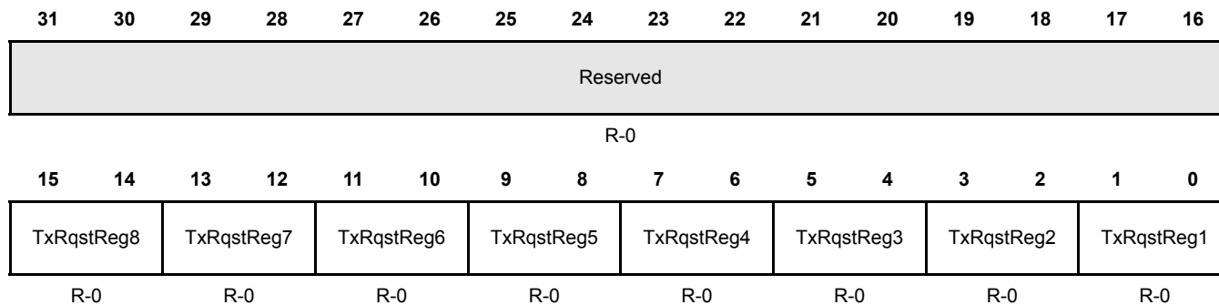
Figure 16-33. Transmission Request X Register (DCAN TXRQ X) [offset = 0x84]
