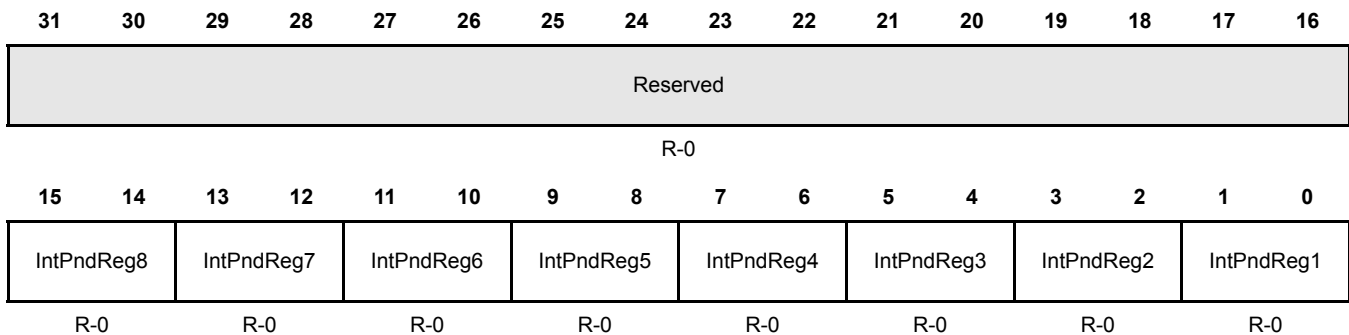
Figure 16-37. Interrupt Pending X Register (DCAN INTPND X) [offset = 0xAC]
