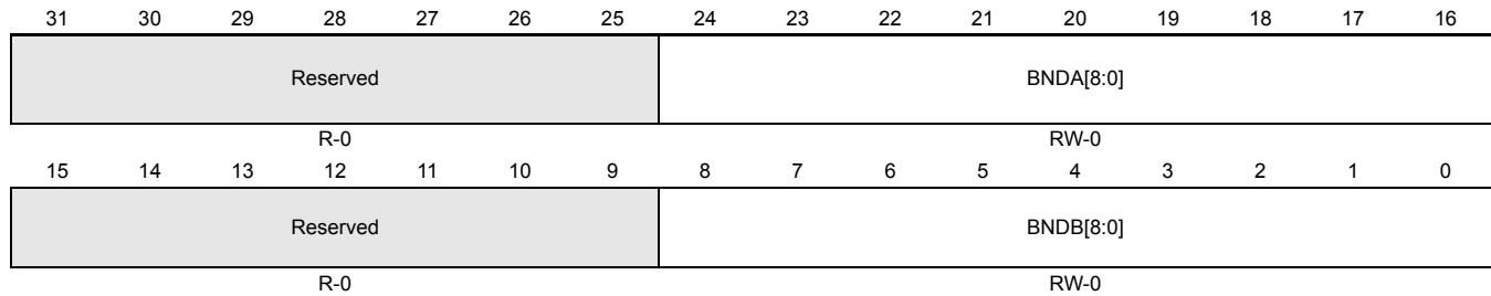
Figure 15-45. ADC Results Memory Configuration Register (ADBNDCCR) [offset = 0x58]
