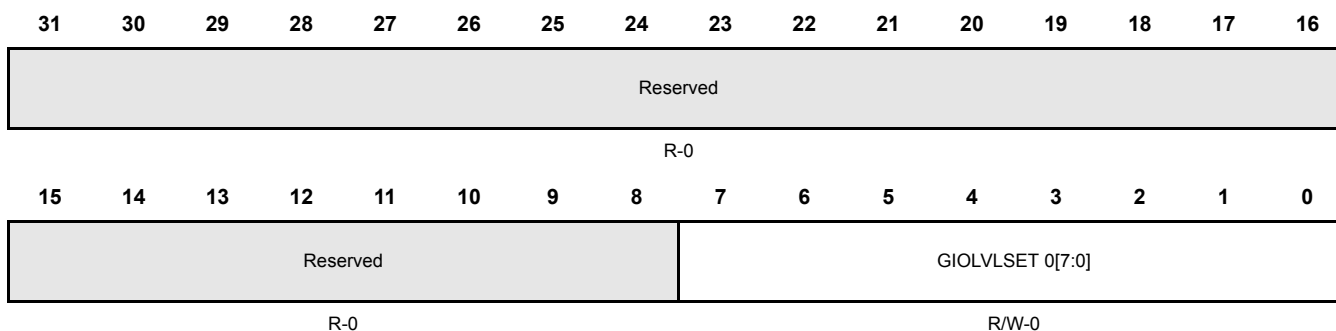
Figure 12-16. GIO Interrupt Priority Register (GIOLVLSET) [0xFFF7BC18]
