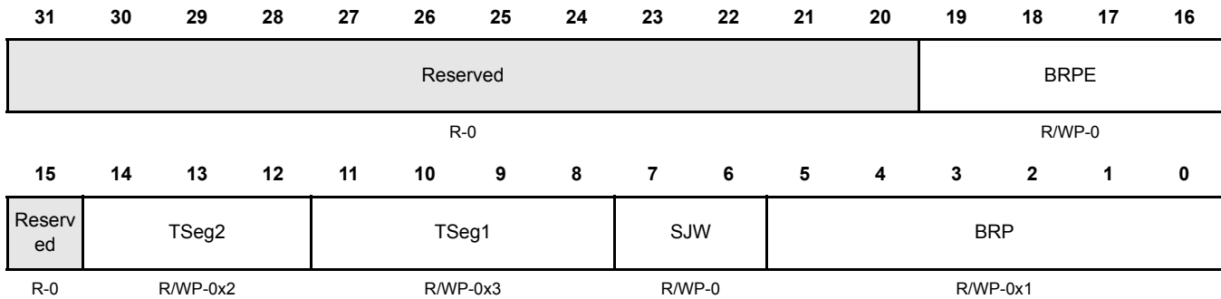
Figure 16-28. Bit Timing Register (DCAN BTR) [offset = 0x0C]
