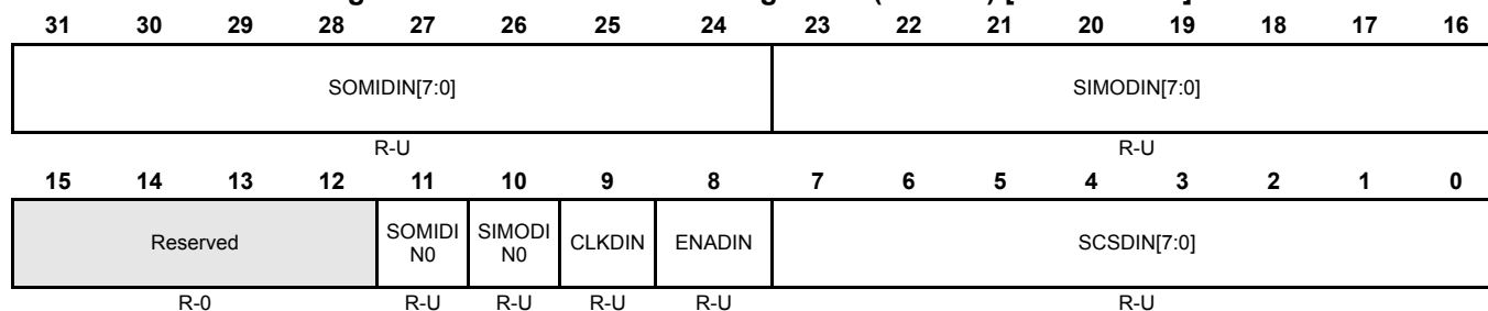
Figure 14-8. SPI Pin Control Register 2 (SPIPC2) [offset = 1Ch]
