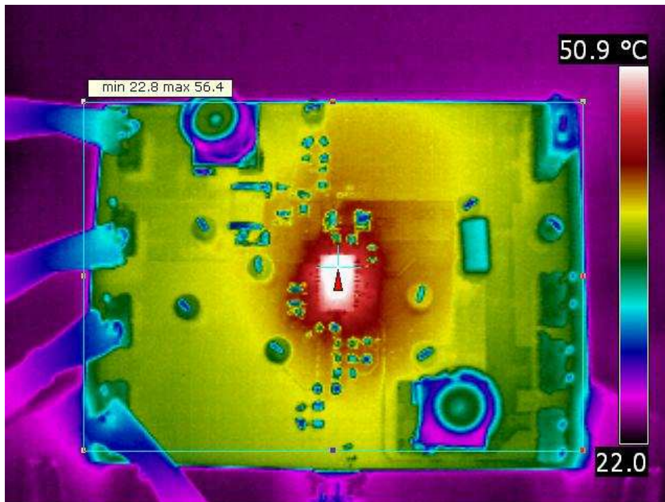
Figure 8. TPS54120 Thermal Image
