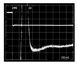
Figure 2. Typical AD684 Hold Mode
