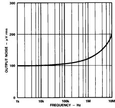
Figure 5. RMS Noise vs. Input Bandwidth of ADC
