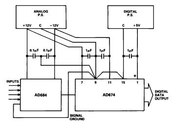
Figure 4. Basic Grounding and Decoupling Diagram
