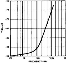
Figure 7. Total Harmonic Distortion vs. Frequency
