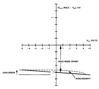
Figure 3. Hold Mode Offset, Gain Error and Nonlinearity
