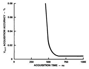
Figure 1. V<sub>OUT</sub> Settling vs. Acquisition Time
