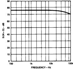
Figure 8. Signal/(Noise and Distortion) vs. Frequency
