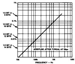
Figure 6. Error Magnitude vs. Frequency
