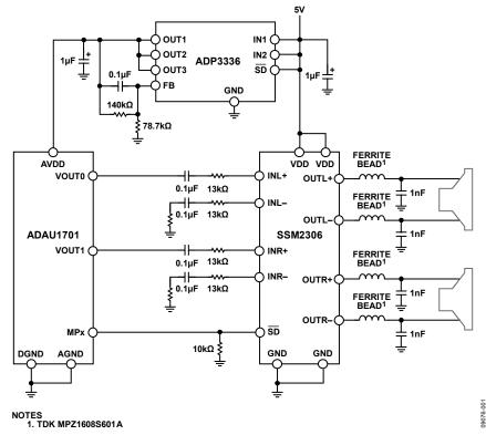
Figure 1. Class-D Amplifier Connection to Audio Codec and Voltage Regulator (Simplified Schematic: Power Supply Decoupling and All Connections Not Shown)
