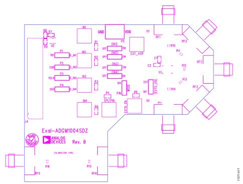
Figure 18. EVAL-ADGM1004SDZ Component Side, Silkscreen PCB Drawing (Top)
