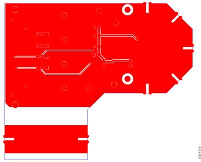
Figure 17. EVAL-ADGM1004SDZ Component Side, Bottom Side PCB Drawing (Layer 4)
