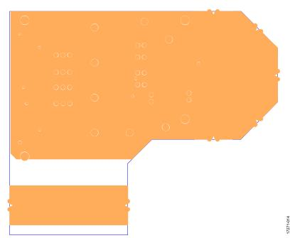
Figure 15. EVAL-ADGM1004SDZ Component Side, Ground Plane PCB Drawing (Layer 2)
