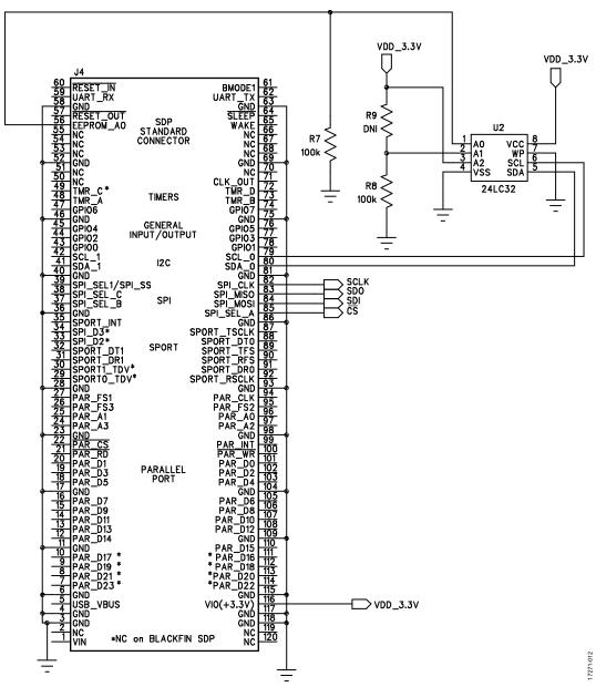
Figure 13. EVAL-ADGM1004SDZ Schematic with SDP-B Board
