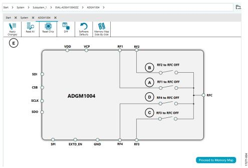
Figure 5. Labeled EVAL-ADGM1004SDZ Block Diagram
