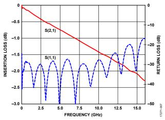
Figure 8. Calibration Transmission Line Insertion Loss (S(2,1)) and Return Loss (S(1,1))
