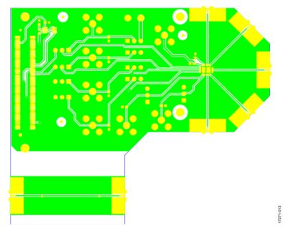
Figure 14. EVAL-ADGM1004SDZ Component Side, PCB Drawing (Layer 1)
