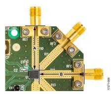
Figure 9. Length of A + B Equal to Length of Calibration Transmission Line
