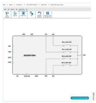
Figure 4. Chip Block Diagram View of the EVAL-ADGM1004SDZ Plugin
