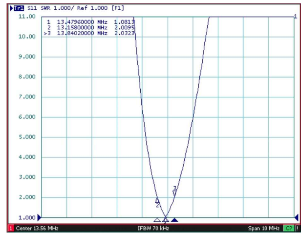
Figure 12. Higher Q Antenna Measurement Plots with Calculated Values ( Q \approx 20 )
