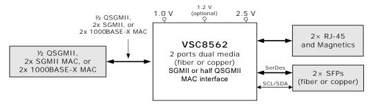
Figure 2 • Copper Transceiver Application Diagram
