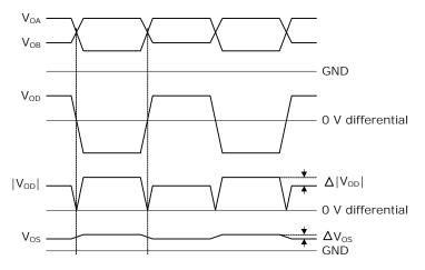
$$\Delta |V_{OD}| = ||V_{OAH} - V_{OBL}| - |V_{OBH} - V_{OAL}||$$
