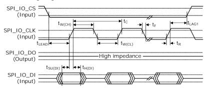
Figure 76 • SI Output Data Timing Diagram for Slave Mode
