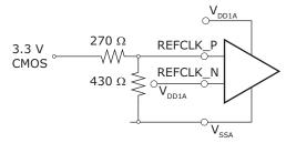
Figure 49 • 5 V CMOS Single-Ended REFCLK Input Resistor Network
