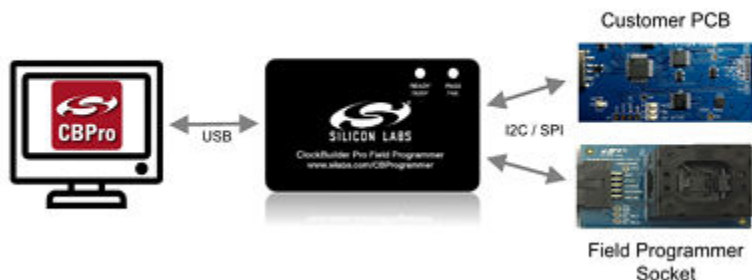
Figure 4.1. PC to CBPROG-DONGLE Connection
